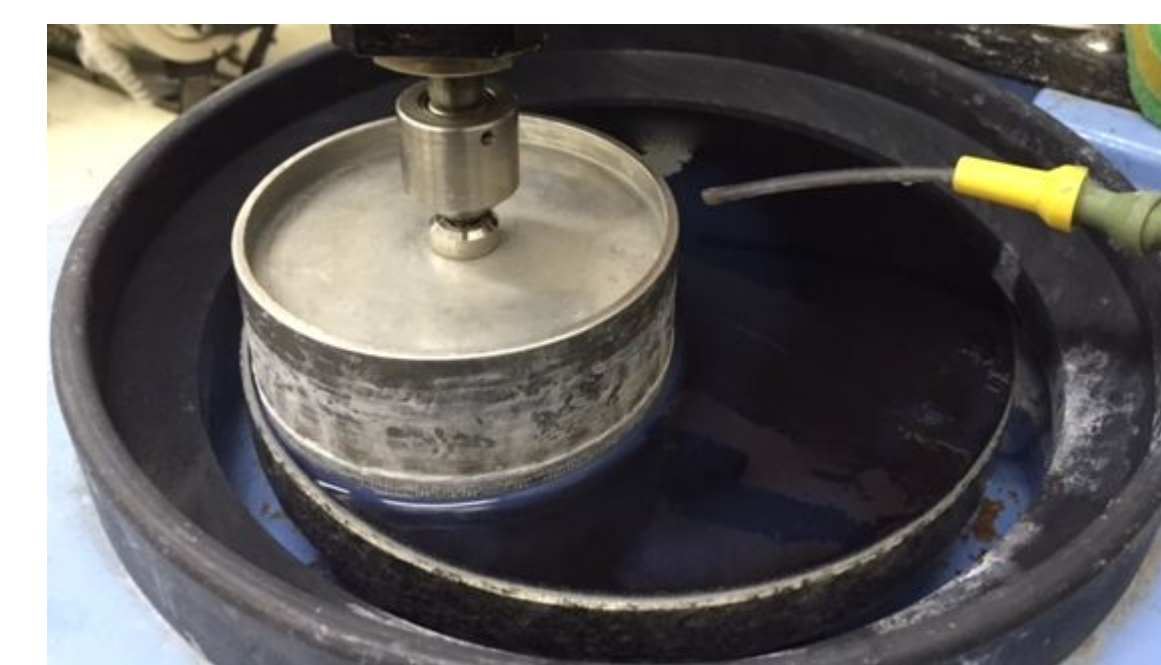
Lapping machine during CMP
