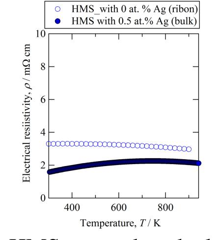
The electrical resistivity of p-type HMS was reduced a lot while the Seebeck coefficient was almost unchanged, both caused by the distributed small Ag.
