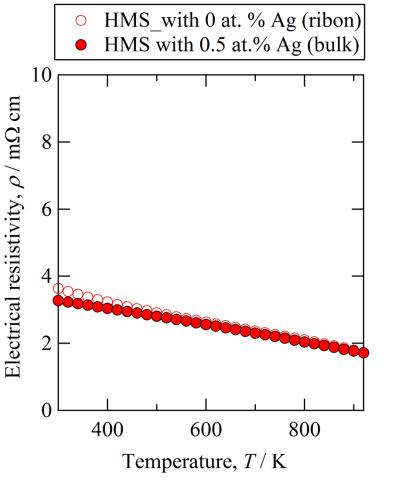
Surprisingly, the electrical resistivity and Seebeck coefficient of n-type HMS were not affected by adding 0.5 at. % Ag.
