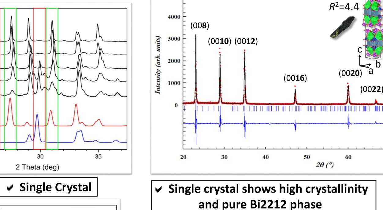
Powder XRD shows only desired (Bi2212) peaks after heating to 865 °C, suggesting a high purity powder
